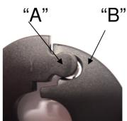
To match the two bearings, rest them on the bar while keeping them slanting so that the protruding part "A" is in front of the hollow part "B", then bring them vertical by a slight pression.
