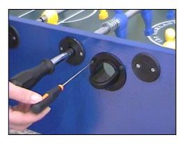
Insert manually the ball entry fillers, insert and tighten the screws into the holes. Do the same with the other ball entry filler.
